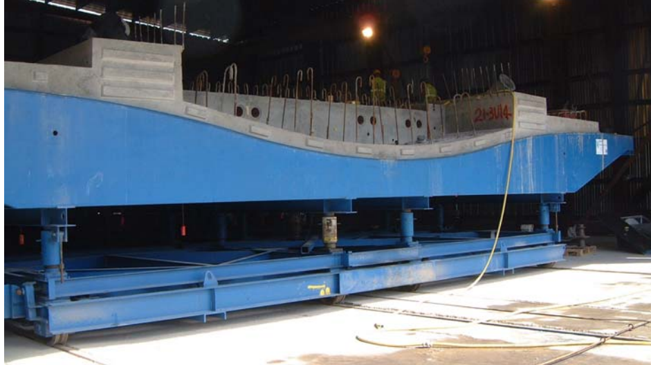
Figure 15 Mould for Precast Shell
